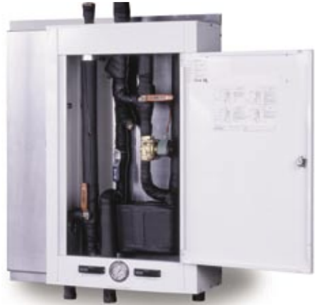
Automatic city water switch over panel includes optional heat exchanger to isolate process liquid/glycol from drain.
