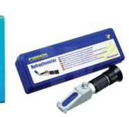
Refractometer to test **Glycol Concentration**
